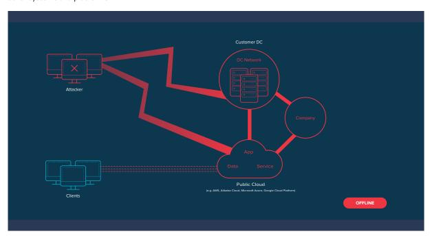
Continuous monitoring of the entire virtual and local IT infrastructure as well as real-time traffic filtering is the best protection against DDoS-related failures. In this process, data traffic is routed through an external filter cluster. In the Scrubbing Center, attacker traffic is separated from legitimate client access.
